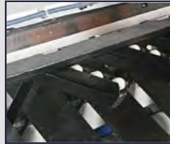
Pnömatik Sac Destek Sistemi Pneumatic Sheet Support
