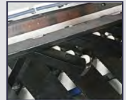
Pnömatik Sac Destek Sistemi Pneumatic Sheet Support
